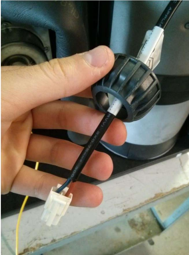
*Take the ring nut, pass it through the cable and screw it in the exchanger gripping the heater's rubber cap.*
