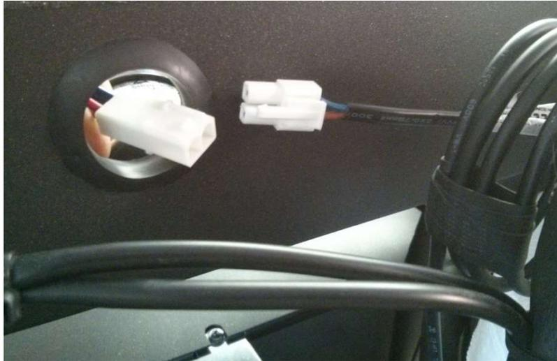
*Connect the heater's connector to thermostat's ones.*
